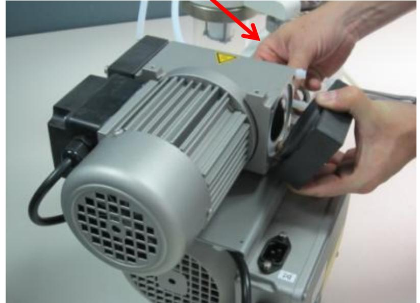
**12. Insert teflon tubing into fitting on head and hand tighten plastic compression nut. Thread 4 bolts to secure heads. Snug tight the 4 bolts. Snug tight the plastic compression nut with 14 mm wrench.**
