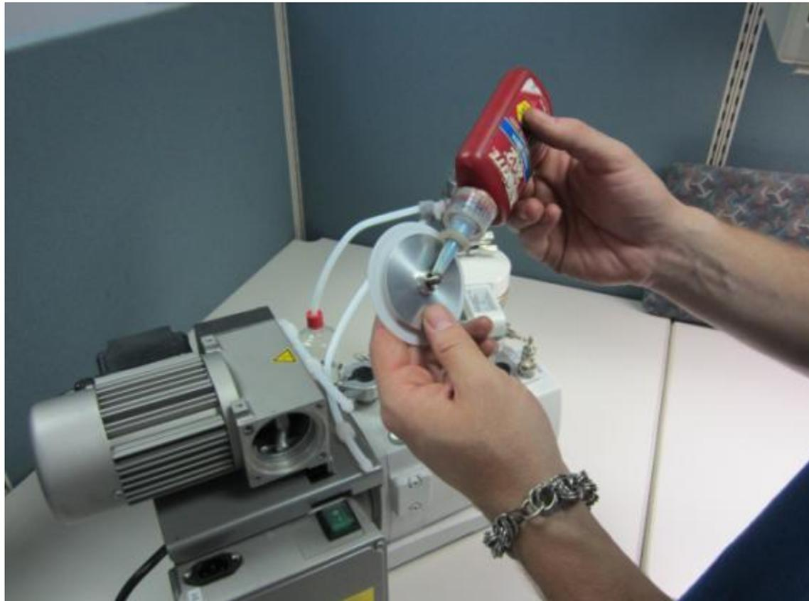
**8. Use spanner to install diaphragm assembly by turning the tightening washer. Make snug.**
