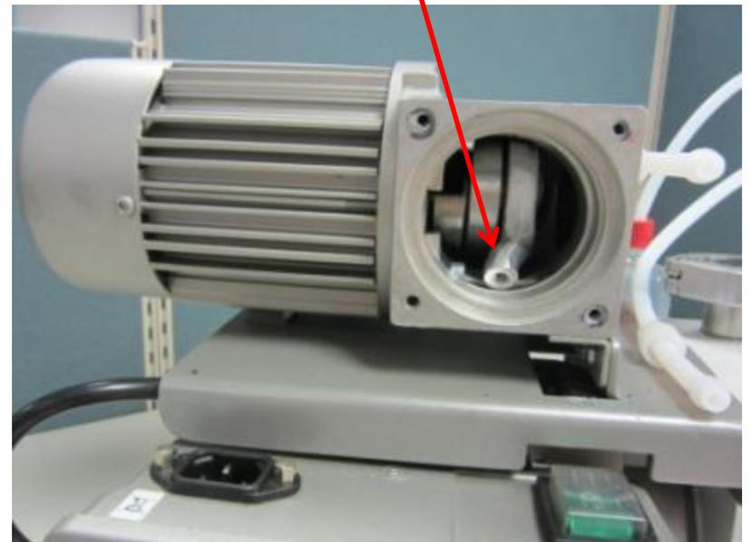
**6. Assembly together diaphragm support plate (pressure washer), new diaphragm and tightening washer (diaphragm holding plate)**
