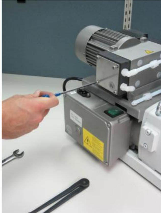
**2. Remove connection head and remove two valves and two o-rings**
